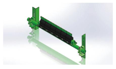
The Belle Banne A -Type secondary belt cleaner has segmented tips that individually adjust to troughs or wear of a belt to apply uniform pressure on the entire width of the belt.
